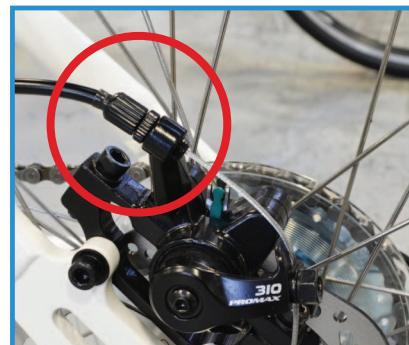
For non-hydraulic brakes a barrel adjuster is situated at the top of the brake caliper, screw the adjuster to tighten the cable.
