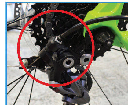
To adjust the rear mech/derailleur, screw the barrel adjuster on the end of the cable housing.
