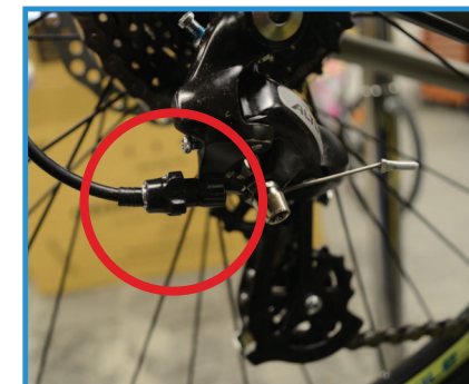
The rear mech/derailleur also has a barrel adjuster which can be used to tighten the cable
