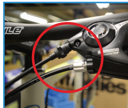
A barrel adjuster is situated on the brake lever and gear shifter. Screw the adjuster to tighten the cables.
